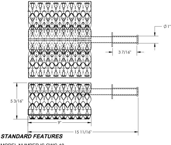
MODEL NUMBER IS GWC-10 OVERALL WIDTH IS 10 7/8" USABLE WIDTH IS 10 7/8" OVERALL LENGTH IS 15 11/16" USABLE LENGTH IS 9" OVERALL HEIGHT IS 5 3/16"
